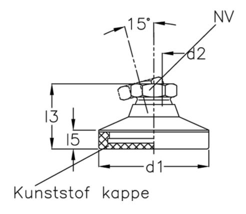
d1 = 40 d2 = 10 l3 = 27.5 l5 = 7.5 NV = 15 Static load (N) = 20 t min = 10.5
